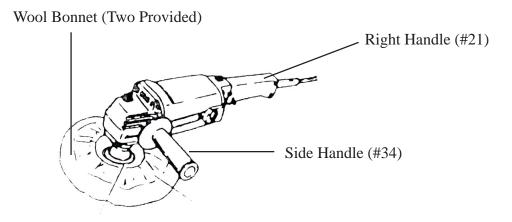
Always hold the **Right Handle** (#21) and the **Side Handle** (#34) firmly when operating the tool. Use Wool Bonnet with a small amount of polishing compound or car wax. Do not put a lot of pressure on the polishing disc. Too much pressure will result in a poor finish and will possibly overload the motor. The weight of the polisher itself is sufficient. Do not wax or polish a car in the direct sunlight. Work in a shaded area.
